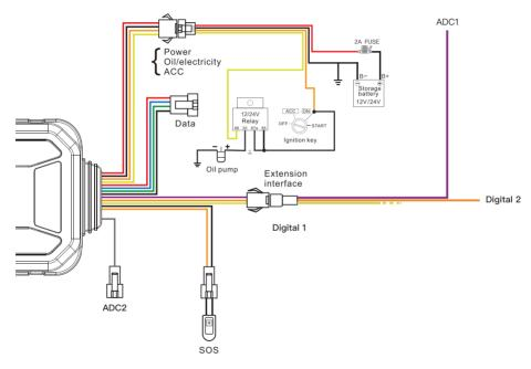
**Notice:** Purple line (ADC) of terminal connects to analog signals line, like voltage of external device, analog temperature sensor, fuel sensor. Voltage detected by analog signal ranges from 0~30Vdc.
